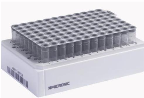
The Micronic TPE Capmat is compatible with 96-well format tubes. The TPE capmat is a sheet of 96 caps with a fixed foil that can be used to seal a full rack of 96 tubes at once. Unlike tubes capped with a TPE capcluster, tubes capped with a TPE capmat cannot be individually removed from the rack—all 96 tubes are capped together. The Micronic TPE cap formats are: the Capcluster-96, the Capmat-96 and the Capband-8 or -12.
